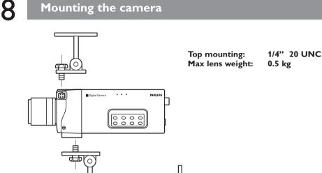
Bottom mounting: 1/4" 20 UNC Max. lens weight: 1.5 kg
